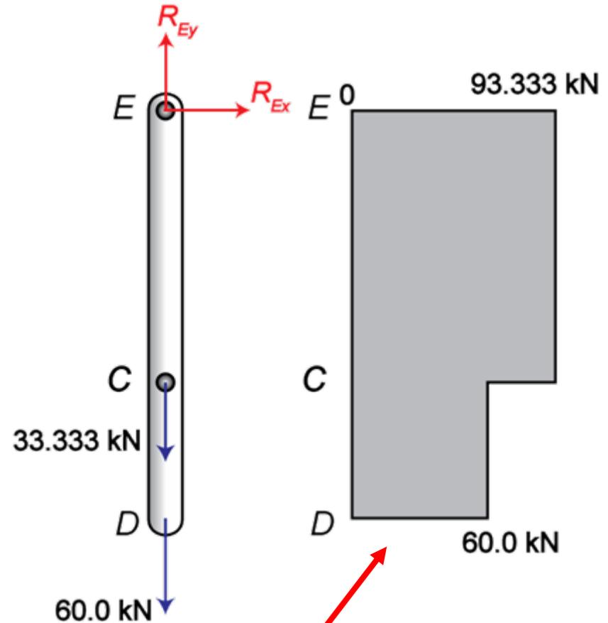
The internal axial force diagram is as shown
