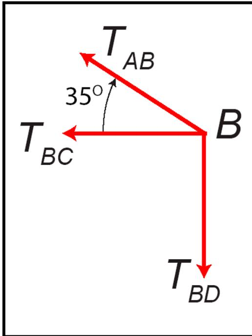
$$\begin{aligned} \sigma_{AB} &= \frac{4378.5 \text{ N}}{\pi \cdot (8.0 \text{ mm})^2 / 4} \\ &= 87.107 \text{ MPa} \end{aligned}$$
